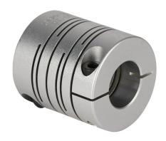
Sung-II Machinery drive coupling, servo-beam, 7075-T6 aluminum alloy, clamp, size 39, 12 x 19mm bore.
