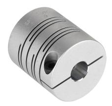
Sung-II Machinery drive coupling, servo-beam, 7075-T6 aluminum alloy, clamp, size 39, 10 x 12mm bore.
