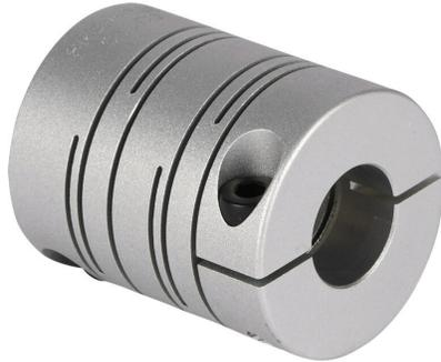
Sung-II Machinery drive coupling, servo-beam, 7075-T6 aluminum alloy, clamp, size 32, 9.525 (3/8in) x 14mm bore.
