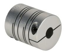
Sung-II Machinery drive coupling, servo-beam, 7075-T6 aluminum alloy, clamp, size 32, 8 x 9.525mm (3/8in) bore.
