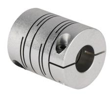
Sung-II Machinery drive coupling, servo-beam, 7075-T6 aluminum alloy, clamp, size 32, 10 x 14mm bore.
