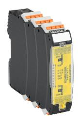
Schmersal safety relay, configurable, 2-channel, 24 VDC, 22 configurations, (2) N.O. and (2) OSSD safety output(s), (1) N.C and (1) status monitoring output(s), push-in cage clamp.
