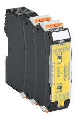
Schmersal safety relay, configurable, release delay, 0 to 30 seconds, 2-channel, 24 VDC, 10 configurations, (3) delayed N.O. and (2) OSSD safety output(s), (1) N.C and (1) status monitoring output(s), push-in cage clamp.
