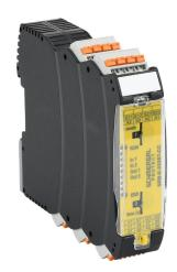
Schmersal safety relay, configurable, release delay, 0 to 30 seconds, 2-channel, 24 VDC, 10 configurations, (3) N.O. and (2) delayed OSSD safety output(s), (1) N.C and (1) status monitoring output(s), push-in cage clamp.
