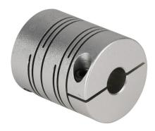
Sung-II Machinery drive coupling, servo-beam, 7075-T6 aluminum alloy, clamp, size 26, 8 x 8mm bore.
