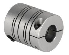
Sung-Il Machinery drive coupling, servo-beam, 7075-T6 aluminum alloy, clamp, size 26, 6.35 (1/4in) x 12mm bore.
