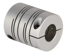
Sung-II Machinery drive coupling, servo-beam, 7075-T6 aluminum alloy, clamp, size 26, 12 x 12mm bore.
