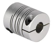
Sung-II Machinery drive coupling, servo-beam, 7075-T6 aluminum alloy, clamp, size 22, 8 x 8mm bore.
