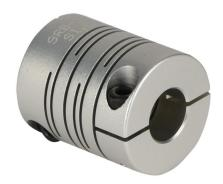
Sung-II Machinery drive coupling, servo-beam, 7075-T6 aluminum alloy, clamp, size 22, 5 x 9.525mm (3/8in) bore.
