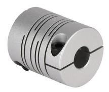
Sung-II Machinery drive coupling, servo-beam, 7075-T6 aluminum alloy, clamp, size 22, 5 x 8mm bore.
