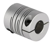
Sung-II Machinery drive coupling, servo-beam, 7075-T6 aluminum alloy, clamp, size 22, 10 x 10mm bore.
