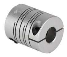
Sung-II Machinery drive coupling, servo-beam, 7075-T6 aluminum alloy, clamp, size 19, 8 x 8mm bore.
