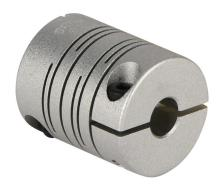
Sung-II Machinery drive coupling, servo-beam, 7075-T6 aluminum alloy, clamp, size 19, 6 x 6mm bore.
