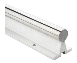
PBC Simplicity 60 Plus series linear precision ground supported shaft, 440C stainless steel, RC50-55, 8-12Ra, 1-1/4in diameter, 24in length. For use with 1-1/4in PBC bearings.
