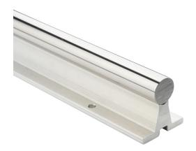
PBC Simplicity 60 Plus series linear precision ground supported shaft, 440C stainless steel, RC50-55, 8-12Ra, 1in diameter, 36in length. For use with 1in PBC bearings.
