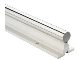
PBC Simplicity 60 Plus series linear precision ground supported shaft, 440C stainless steel, RC50-55, 8-12Ra, 1in diameter, 24in length. For use with 1in PBC bearings.
