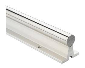
PBC Simplicity 60 Plus series linear precision ground supported shaft, 440C stainless steel, RC50-55, 8-12Ra, 1in diameter, 12in length. For use with 1in PBC bearings.
