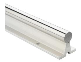
PBC Simplicity 60 Plus series linear precision ground supported shaft, 1060 steel, RC60-65, 8-12Ra, 1in diameter, 24in length. For use with 1in PBC bearings.
