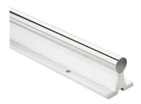
PBC Simplicity 60 Plus series linear precision ground supported shaft, 440C stainless steel, RC50-55, 8-12Ra, 3/4in diameter, 12in length. For use with 3/4in PBC bearings.
