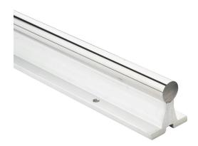
PBC Simplicity 60 Plus series linear precision ground supported shaft, 1060 steel, RC60-65, 8-12Ra, 3/4in diameter, 36in length. For use with 3/4in PBC bearings.
