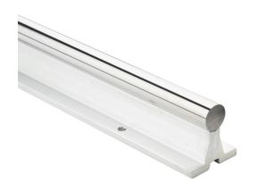
PBC Simplicity 60 Plus series linear precision ground supported shaft, 1060 steel, RC60-65, 8-12Ra, 3/4in diameter, 24in length. For use with 3/4in PBC bearings.
