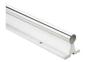
PBC Simplicity 60 Plus series linear precision ground supported shaft, 1060 steel, RC60-65, 8-12Ra, 3/4in diameter, 12in length. For use with 3/4in PBC bearings.
