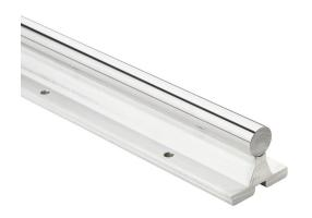
PBC Simplicity 60 Plus series linear precision ground supported shaft, 440C stainless steel, RC50-55, 8-12Ra, 5/8in diameter, 24in length. For use with 5/8in PBC bearings.
