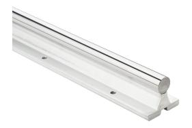
PBC Simplicity 60 Plus series linear precision ground supported shaft, 440C stainless steel, RC50-55, 8-12Ra, 5/8in diameter, 12in length. For use with 5/8in PBC bearings.
