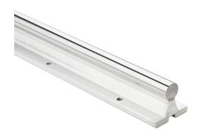
PBC Simplicity 60 Plus series linear precision ground supported shaft, 1060 steel, RC60-65, 8-12Ra, 5/8in diameter, 36in length. For use with 5/8in PBC bearings.
