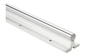
PBC Simplicity 60 Plus series linear precision ground supported shaft, 1060 steel, RC60-65, 8-12Ra, 5/8in diameter, 24in length. For use with 5/8in PBC bearings.
