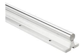
PBC Simplicity 60 Plus series linear precision ground supported shaft, 1060 steel, RC60-65, 8-12Ra, 5/8in diameter, 12in length. For use with 5/8in PBC bearings.
