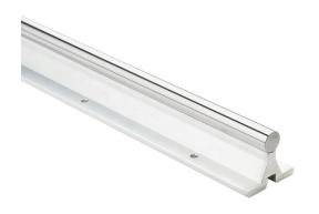
PBC Simplicity 60 Plus series linear precision ground supported shaft, 440C stainless steel, RC50-55, 8-12Ra, 1/2in diameter, 36in length. For use with 1/2in PBC bearings.
