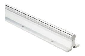
PBC Simplicity 60 Plus series linear precision ground supported shaft, 440C stainless steel, RC50-55, 8-12Ra, 1/2in diameter, 24in length. For use with 1/2in PBC bearings.
