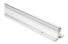
PBC Simplicity 60 Plus series linear precision ground supported shaft, 1060 steel, RC60-65, 8-12Ra, 1/2in diameter, 36in length. For use with 1/2in PBC bearings.
