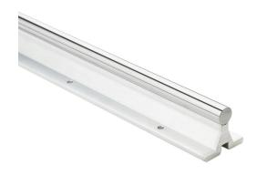
PBC Simplicity 60 Plus series linear precision ground supported shaft, 1060 steel, RC60-65, 8-12Ra, 1/2in diameter, 24in length. For use with 1/2in PBC bearings.
