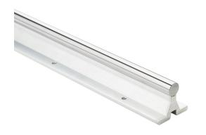
PBC Simplicity 60 Plus series linear precision ground supported shaft, 1060 steel, RC60-65, 8-12Ra, 1/2in diameter, 12in length. For use with 1/2in PBC bearings.
