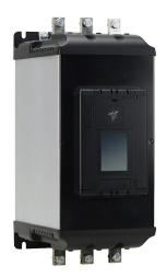
Stellar SR55 series full-featured soft starter, 414A, 200-480 VAC at 3-phase, Trip Class 10/20/30, rated for 3 start/hour, internally bypassed. Optional EtherNet/IP and Modbus TCP cards available.
