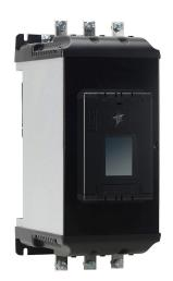
Stellar SR55 series full-featured soft starter, 242A, 200-480 VAC at 3-phase, Trip Class 10/20/30, rated for 3 start/hour, internally bypassed, 3 frame. Optional EtherNet/IP and Modbus TCP cards available.
