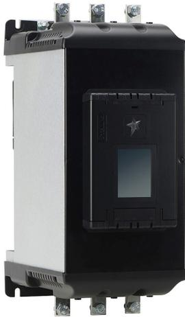
Stellar SR55 series full-featured soft starter, 242A, 200-480 VAC at 3-phase, Trip Class 10/20/30, rated for 3 start/hour, internally bypassed, 3 frame. Optional EtherNet/IP and Modbus TCP cards available.
