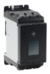
Stellar SR55 series full-featured soft starter, 180A, 200-480 VAC at 3-phase, Trip Class 10/20/30, rated for 3 start/hour, internally bypassed. Optional EtherNet/IP and Modbus TCP cards available.
