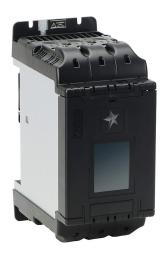
Stellar SR55 series full-featured soft starter, 156A, 200-480 VAC at 3-phase, Trip Class 10/20/30, rated for 5 start/hour, internally bypassed, 2 frame. Optional EtherNet/IP and Modbus TCP cards available.
