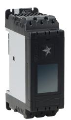
Stellar SR55 series full-featured soft starter, 96A, 200-480 VAC at 3-phase, Trip Class 10/20/30, rated for 5 start/hour, internally bypassed. Optional EtherNet/IP and Modbus TCP cards available.
