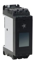
Stellar SR55 series full-featured soft starter, 65A, 200-480 VAC at 3-phase, Trip Class 10/20/30, rated for 5 start/hour, internally bypassed. Optional EtherNet/IP and Modbus TCP cards available.
