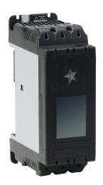
Stellar SR55 series full-featured soft starter, 52A, 200-480 VAC at 3-phase, Trip Class 10/20/30, rated for 5 start/hour, internally bypassed. Optional EtherNet/IP and Modbus TCP cards available.
