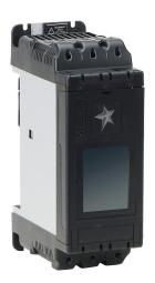
Stellar SR55 series full-featured soft starter, 34A, 200-480 VAC at 3-phase, Trip Class 10/20/30, rated for 5 start/hour, internally bypassed, 1 frame. Optional EtherNet/IP and Modbus TCP cards available.
