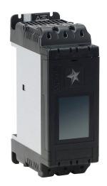
Stellar SR55 series full-featured soft starter, 27A, 200-480 VAC at 3-phase, Trip Class 10/20/30, rated for 5 start/hour, internally bypassed. Optional EtherNet/IP and Modbus TCP cards available.
