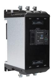
Stellar SR35 series basic soft starter, 302A, 110-240 VAC at 1-phase/208-460 VAC at 3-phase, Trip Class 10/20/30, rated for 3 start/hour, internally bypassed, 3 frame.
