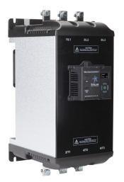
Stellar SR35 series basic soft starter, 242A, 110-240 VAC at 1-phase/208-460 VAC at 3-phase, Trip Class 10/20/30, rated for 3 start/hour, internally bypassed, 3 frame.
