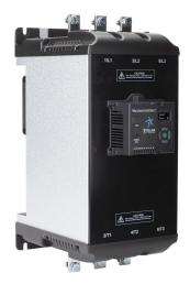
Stellar SR35 series basic soft starter, 242A, 110-240 VAC at 1-phase/208-460 VAC at 3-phase, Trip Class 10/20/30, rated for 3 start/hour, internally bypassed.
