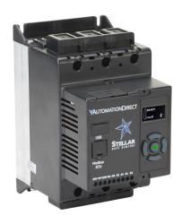
Stellar SR35 series basic soft starter, 65A, 110-240 VAC at 1-phase/208-460 VAC at 3-phase, Trip Class 10/20/30, rated for 5 start/hour, internally bypassed.
