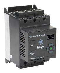
Stellar SR35 series basic soft starter, 41A, 110-240 VAC at 1-phase/208-460 VAC at 3-phase, Trip Class 10/20/30, rated for 5 start/hour, internally bypassed.
