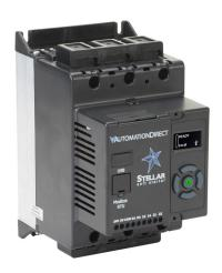
Stellar SR35 series basic soft starter, 34A, 110-240 VAC at 1-phase/208-460 VAC at 3-phase, Trip Class 10/20/30, rated for 5 start/hour, internally bypassed.
